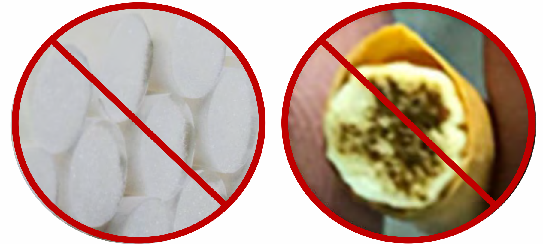
Filters made with Closed C tow are less prone to show recess (left) and hot/wet collapse (right).
