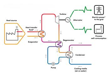
\*Indicates where heat transfer fluid is located in the ORC process. ORC process units can produce electricity and/or mechanical power.
